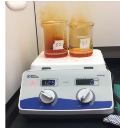
Image 1: Reaction between Sulfuric Acid and Nitric Acid used for digestion
