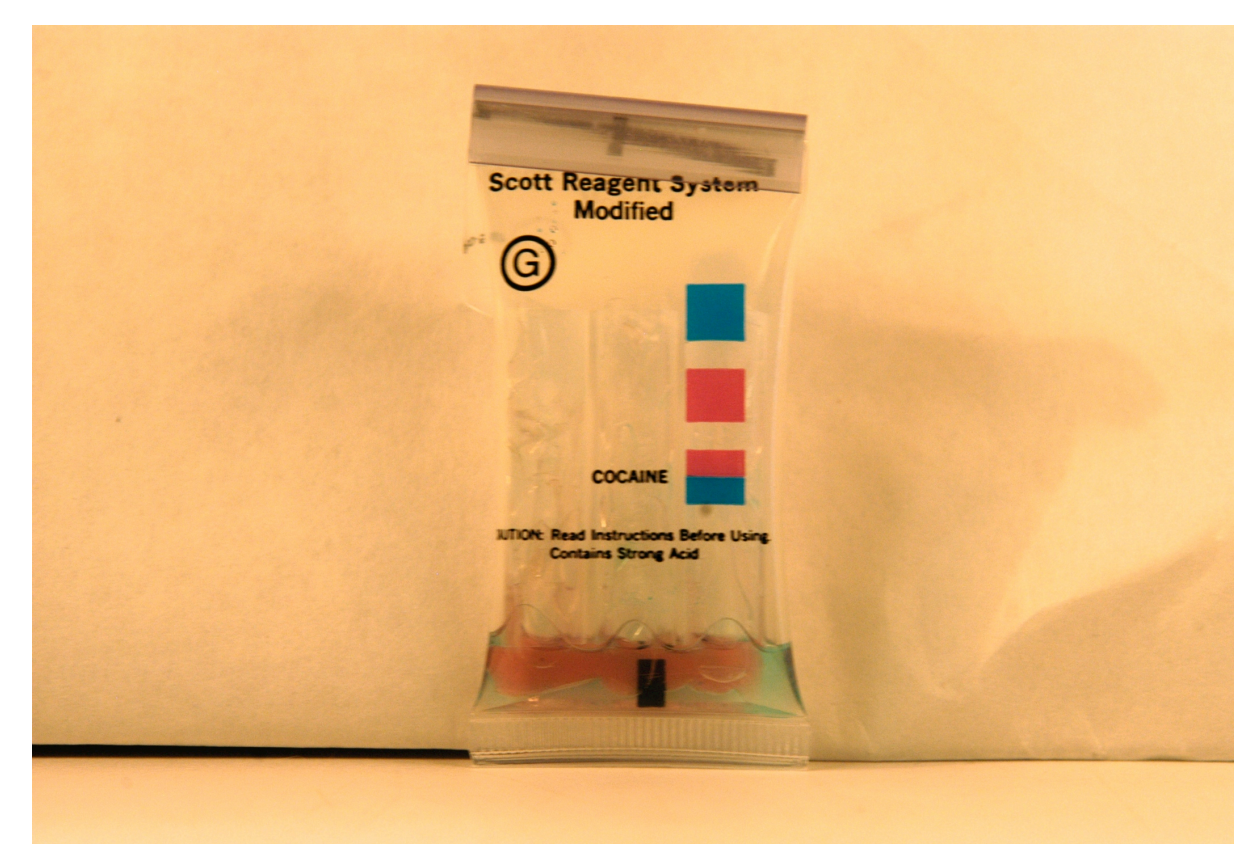
Figure 4: A weaker positive result for cocaine HCl from a mixture that was 10% cocaine and 90% Mannitol.
