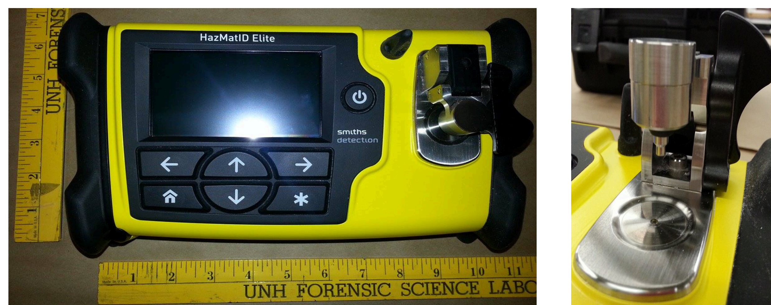
Figure 1 : The HazMatID Elite Portable Infrared Spectrometer (left) and the diamond ATR sampling platform. (pictures courtesy of C. M. Dupper)
