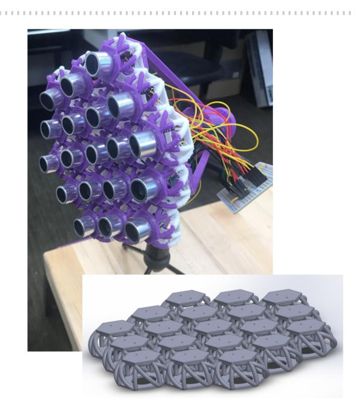
To create a conformal array the ultrasonic transducers must be mounted on a flexible backplane. We used a 3D printer to rapidly iterate upon a NASA-inspired hexagonal fabric design<sup>1</sup>. The radius of curvature of this structure can be varied to change the geometrical focal distance.
