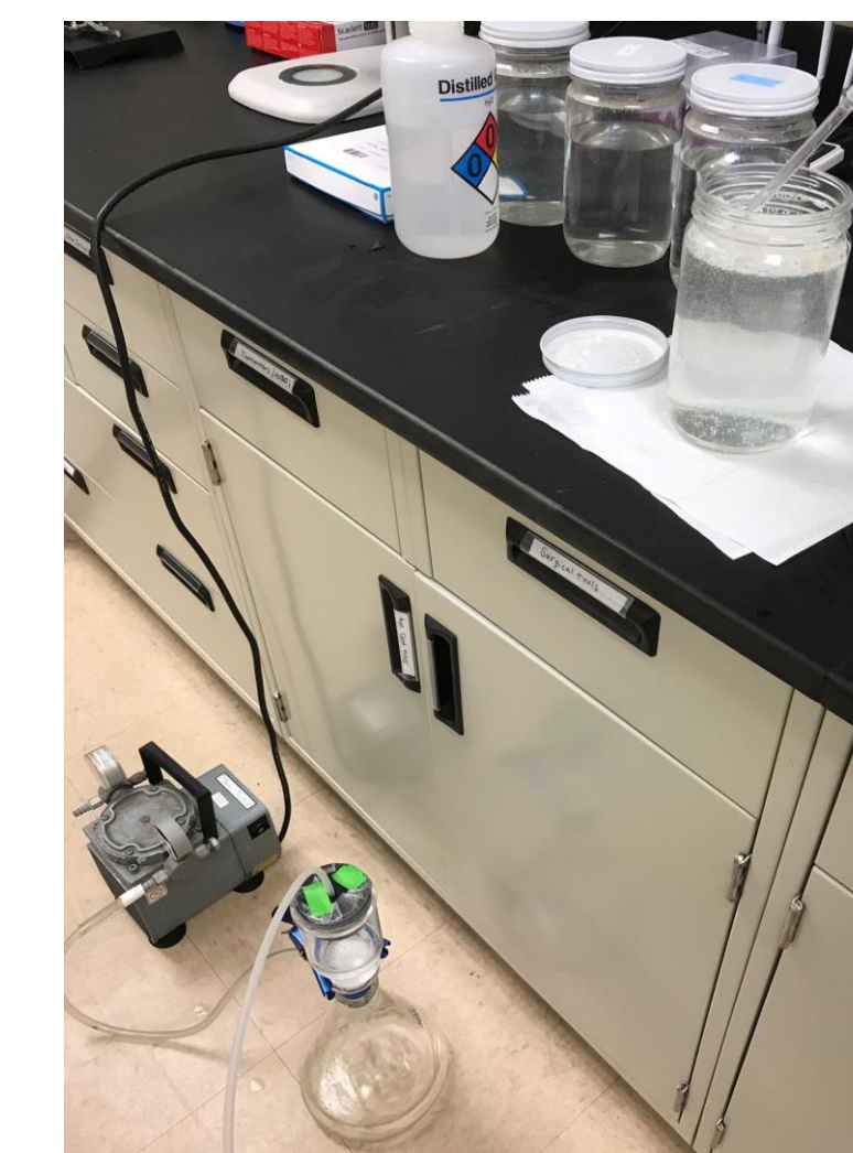
Figure 3 The suctioning apparatus constructed to collect MPs from the samples.
