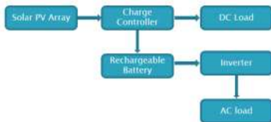
Fig.5. Block Diagram of Stand-alone PV System with Battery Storage
