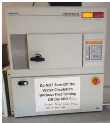
Figure 2: The X-ray Diffractometer used for this project.
