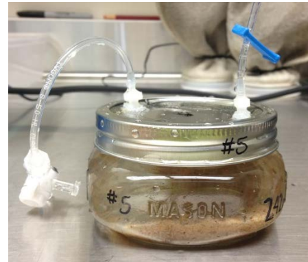
Figure 2: example of the experimental respirometer chambers.
