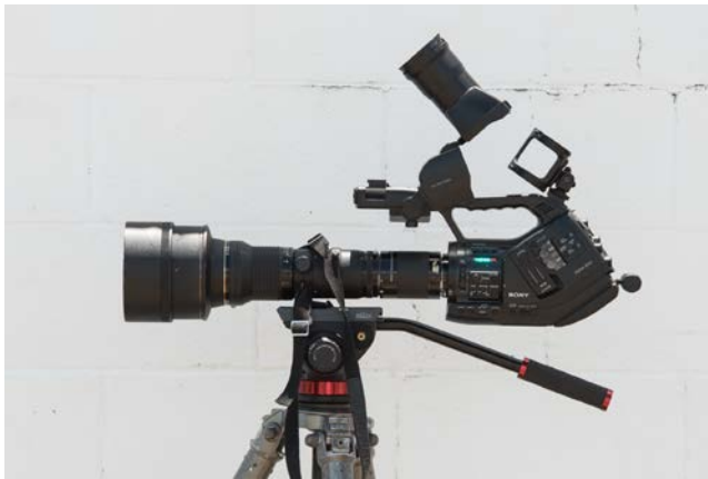
Figure 3: Sony EX3 HD camcorder equipped with Nikon 400mm super telephoto lens and 2x teleconverter.
