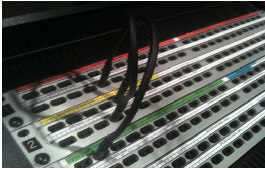
Figure 1 illustrates the patching of the output of the DAW into the input of the preamp and the output of the preamp back into the DAW.
