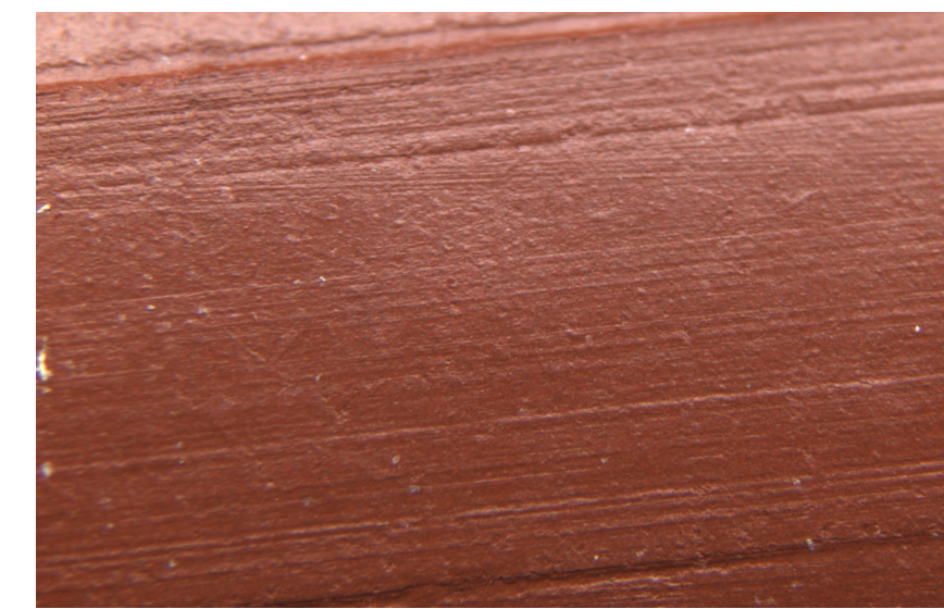
Figure 2: Mikrosil casting of .40 caliber fired bullet from Figure 1. It is a negative image of the same land of the fired bullet.
