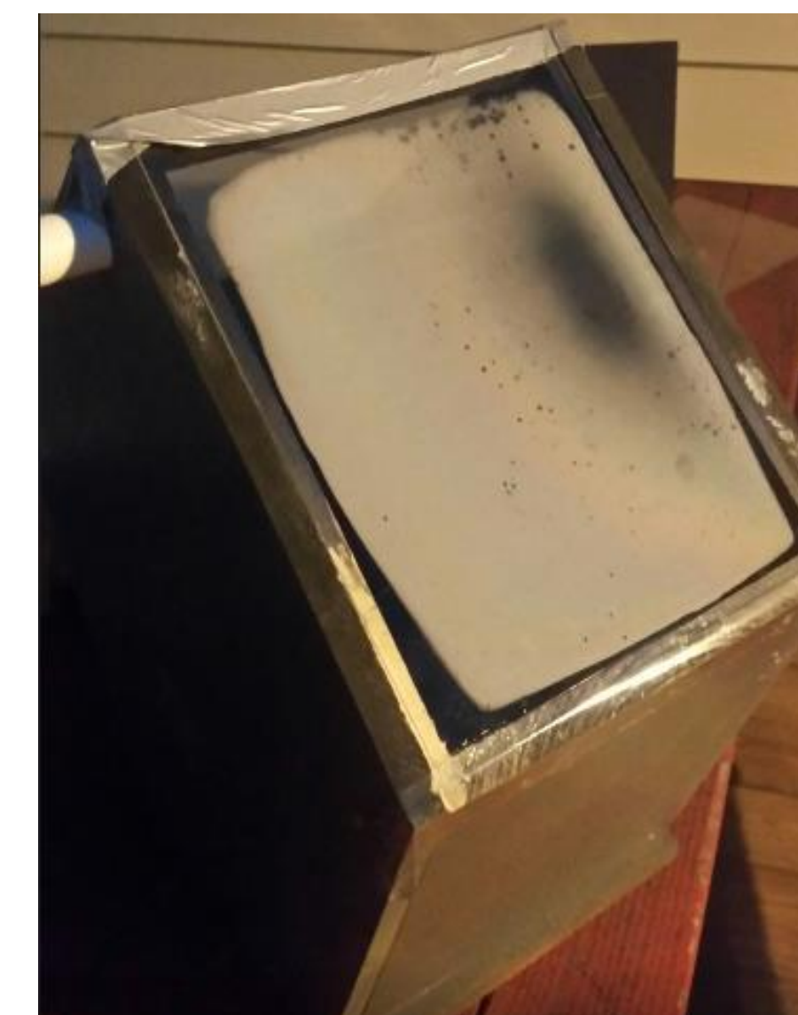
Figure 4 – Prototype condensate collector with condensation
