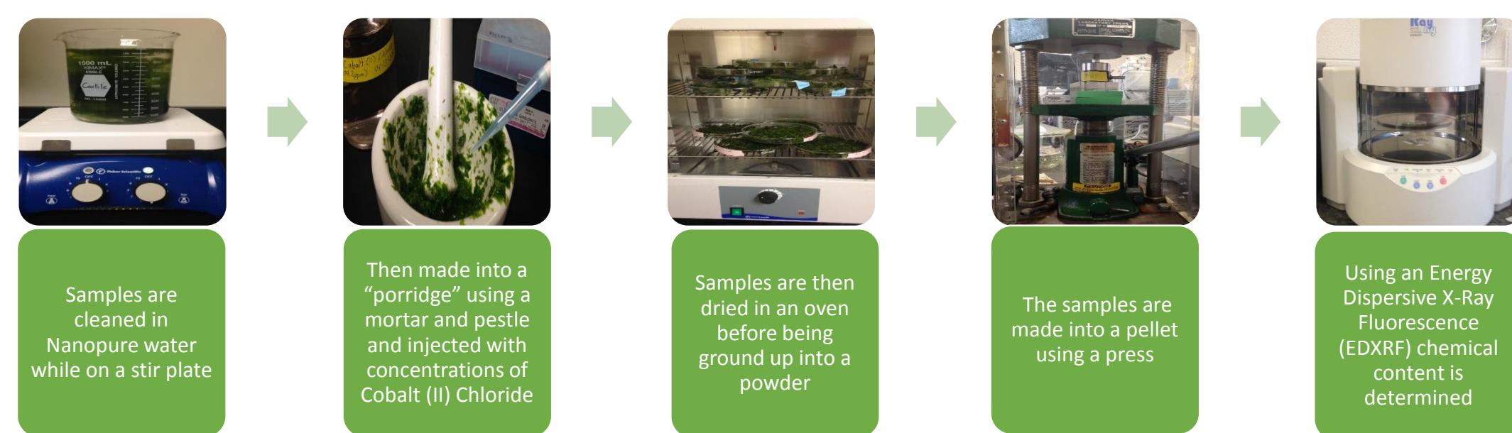
Figure 3 Method of preparing ulvoid samples for EDXRF testing.
