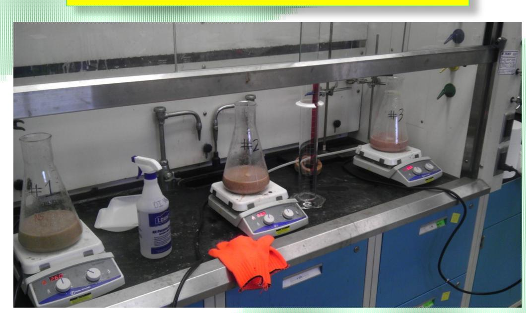
The final step is to remove the ethanol from the fermented mash via distillation. The distillate is then analyzed on a gas chromatogram flame ionization detector.
